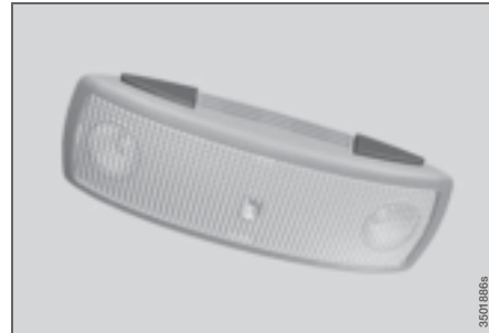
Rear roof lighting
